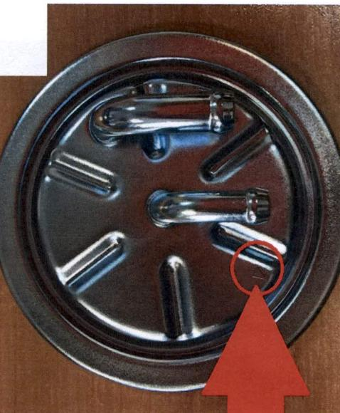
Please scrap the filters with a triangle on retainer as visible on pictures.
